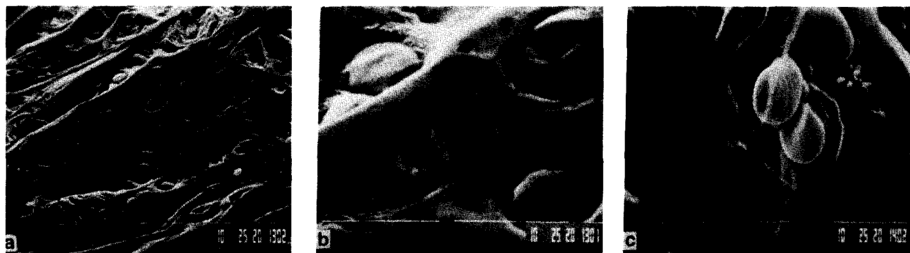
Figure 10 Etched surface of a 10% LCP blend: (a) 1000×, (b) 5000×, (c) 5000×
